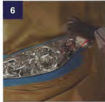
6 Apply SprayMax Headlightprimer with one spray pass until a full wet and opaque dull film is created.
