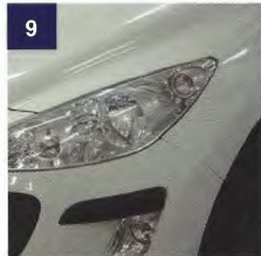
9 Drying: at 20°C/68°F room temperature overnight / or accelerated dry time by using a heat lamp at 60°C/140°F for 15min.
