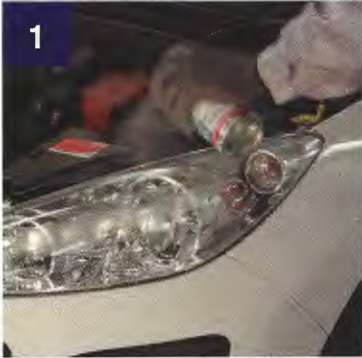
1 Clean thoroughly with SprayMax Wax & Grease Remover
