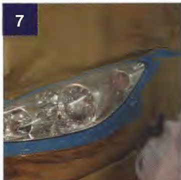
7 Allow a 40 minutes flash off time at 20°C/68°F room temperature. Primer will have a milk white appearance when first applied, when primer is dry it will have a more mat transparent appearance.
