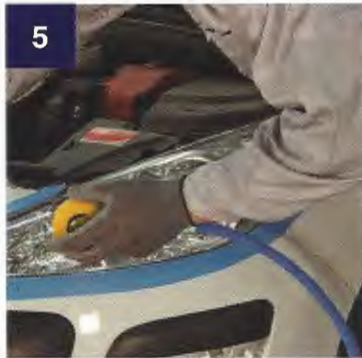
5 Final sanding plastic lens manually with P3000 wet. Clean and dry lens with SprayMax Wax & Grease Remover
