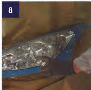
8 First Application of SprayMax Headlight Clear Coat should be a very thin layer (misty), directly followed by a continuous, film-forming spray pass – no flash-off time required!
